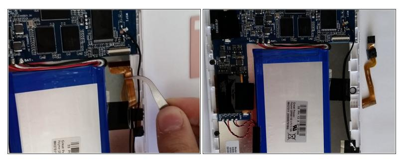
• Remove the orange camera strip from the motherboard.
