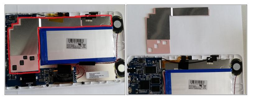
Remove the pink and aluminum protective cover. Be sure to also remove any tape holding it in place.
