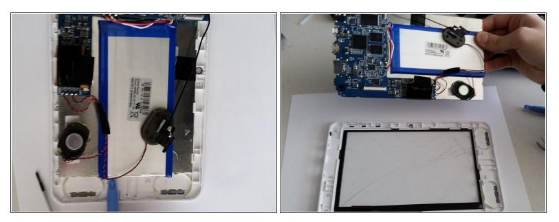
• Pry under the aluminum touch screen to remove the remaining components from the front housing.
