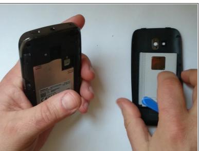
Switch off the phone and remove the battery.
