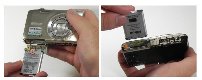
Insert new battery with the arrow facing you or the front of camera.
