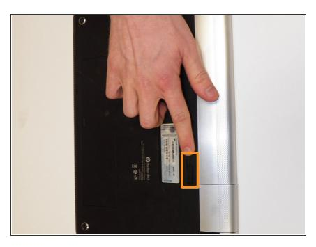
Flip laptop to bottom side and locate the battery eject switch.
