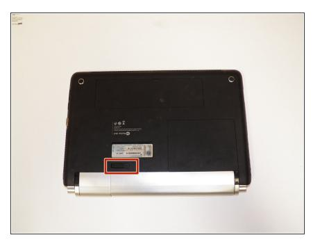
Place the laptop upside down on a stable surface and locate the battery ejection switch.
