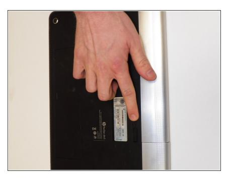
Eject the battery by sliding the switch sideways.
