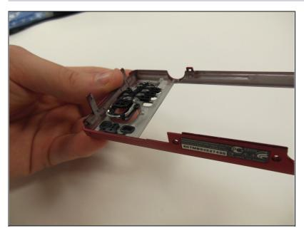
• Carefully pick up frame and push upward on buttons.
