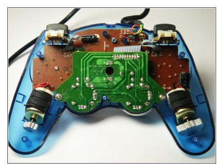
• Remove the two 7 mm screws on the closest circuit board.
