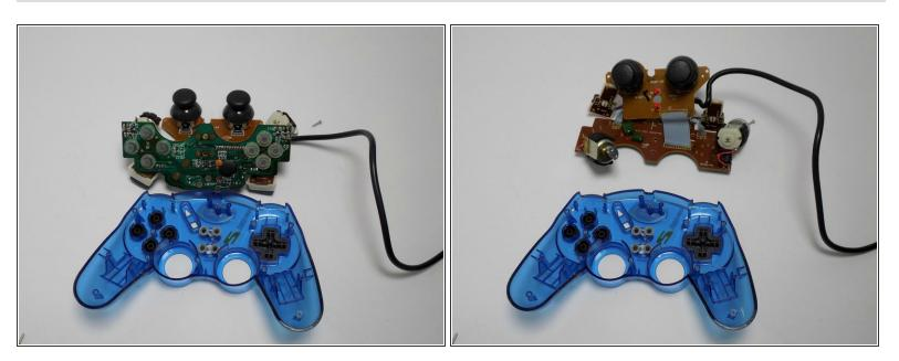
• Remove the motherboard assembly from the cover.
