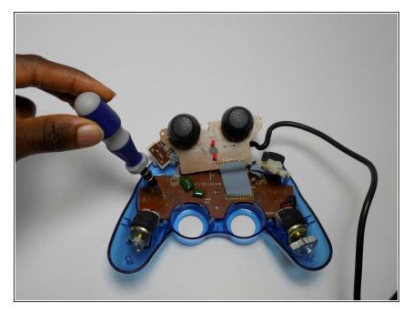
• Remove the two 7 mm Philip screws on the larger circuit board.
