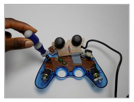
• Remove the two 7 mm Philip screws on the motherboard.
