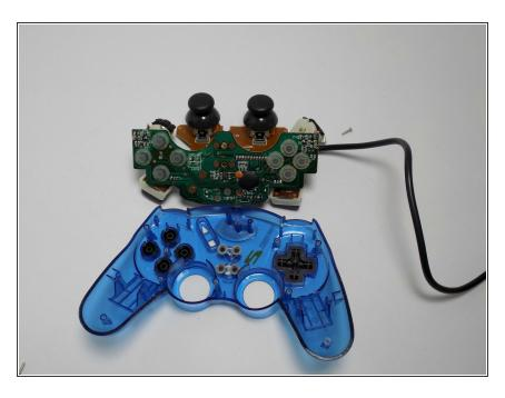
• Remove the motherboard assembly from the cover.
