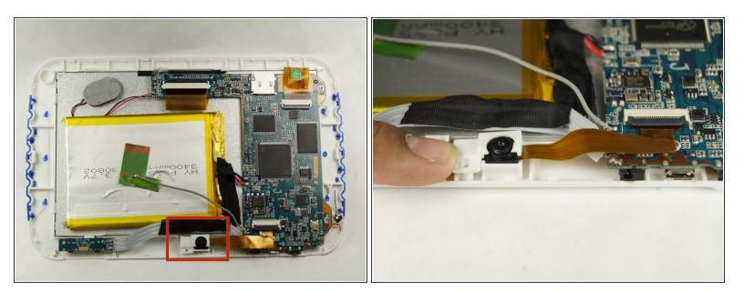
• Locate the camera in the top of the device. Note the plastic clip holding it in place.
