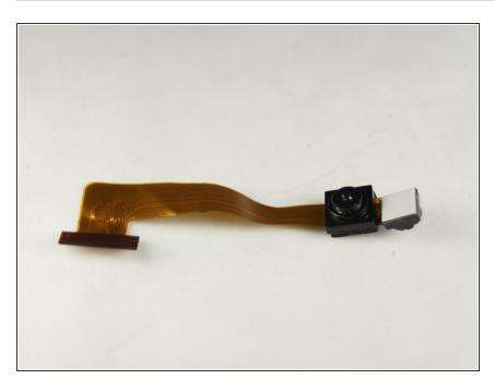
• Take the new camera piece and insert the data cable connection into the connection.
