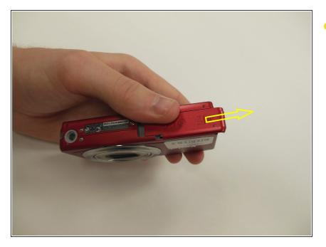
• Push down and slide as indicated on the battery latch.
