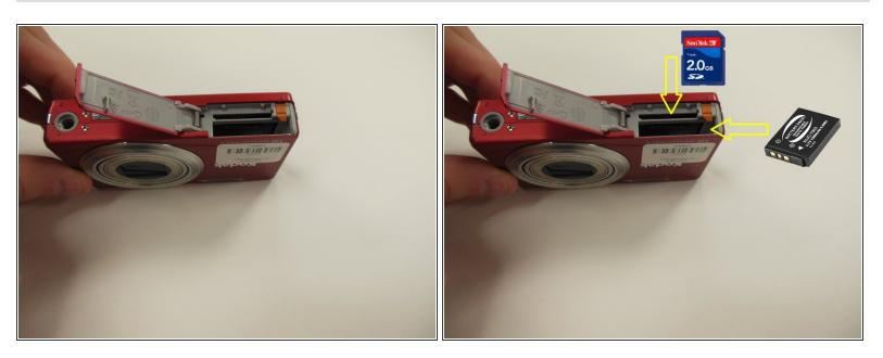
• Push in on the SD Card until it clicks and releases. Remove SD Card.
