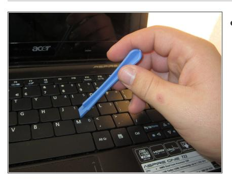
Use plastic opening tool to remove the key.
