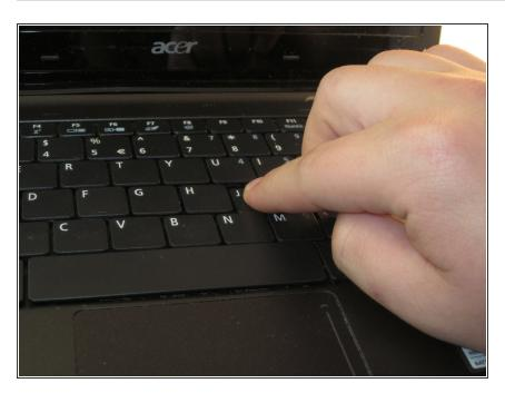
Push working key back into place until it clicks. Make sure key is in correct position.
