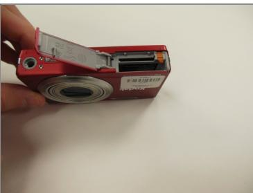
First, press in and slide forward the battery latch as indicated by the arrow.
