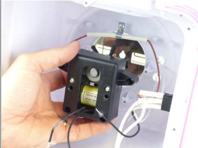
• Line up the prongs on the motor shaft with the holes in the heating element and pull the motor out.
