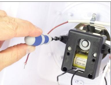
Remove the four 12mm Phillips #02 screws to free the motor housing.
