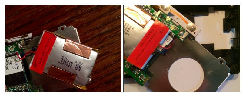
• This is a defective battery. Replace it with a new one.
