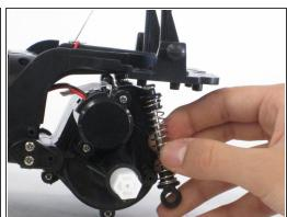
Pull the black washer inside the spring downwards and towards the truck's rear simultaneously in order to remove the suspension.
