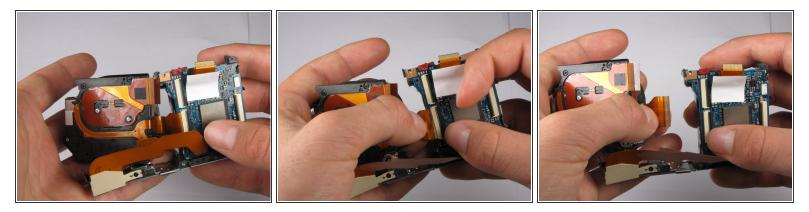
• Disconnect the top remaining ribbon-wire by carefully pulling at the base of where the wire connects to the motherboard.
