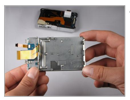
• Pull the LCD and its casing away from the rest of the camera.
