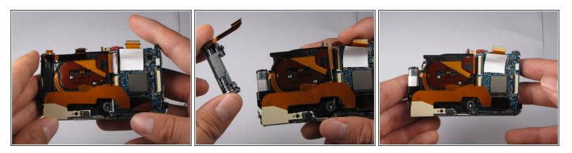
Flash capacitors are dangerous! Be *extremely* careful when removing the capacitor from the camera. You can get shocked *BADLY*!
