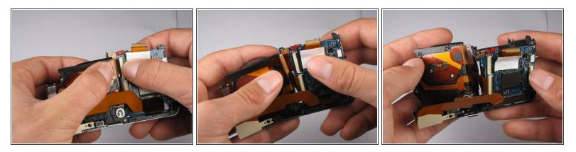
• Carefully disconnect the top ribbon-wire from the motherboard by pulling where the wire connects to the motherboard.
