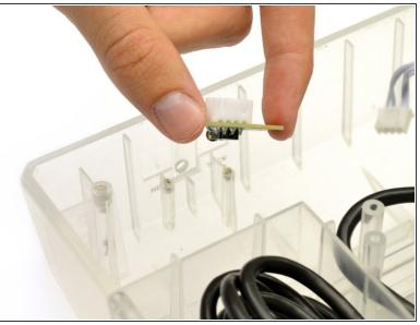
Gently wiggle the headphone jack left and right, pulling it towards you until it slides out of the hole in the enclosure.
