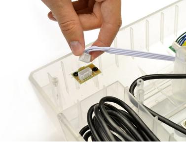
• Grasp the white plug connecting the wires to the headphone jack, and pull gently upwards.
