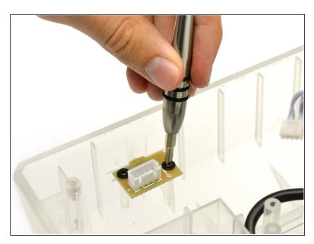
Using a Phillips head #1 screwdriver, remove the two washer head screws from the headphone jack.
