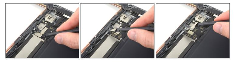
• Use the flat end of a spudger or a fingernail to carefully pop the two digitizer cable connectors straight up from their sockets.
