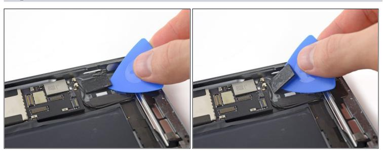
i The SIM board is held to the rear case with a thick adhesive pad.
