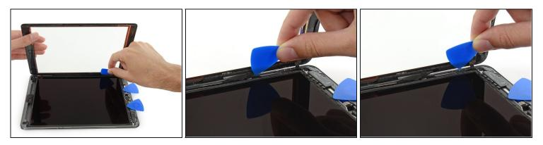
• While supporting the front panel glass, use an opening pick to cut the last of the adhesive.
