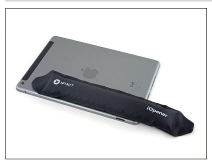
Place a heated iOpener over the SIM tray side of the iPad, and let it sit for at least a minute to soften the adhesive through the rear case.
