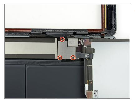
• Remove the three 1.4 mm Phillips screws securing the display cable bracket.
