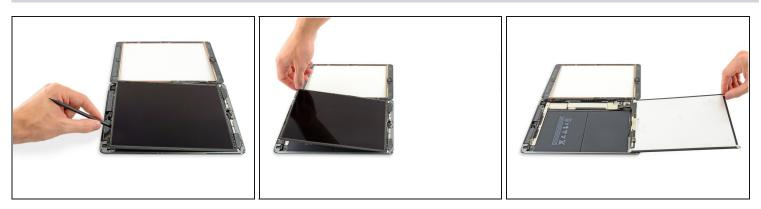
🛆 Do not attempt to fully remove the LCD. It is still connected to the iPad by several cables at the home button end. Lift only from the front-facing camera end.
