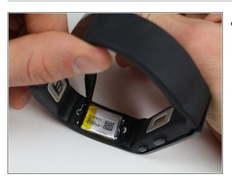
Gently pry up one edge of the battery with the plastic spudger.
