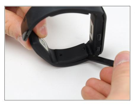
Firmly pry up the side panel using the plastic spudger to break the waterproof seal and lift the battery panel.
