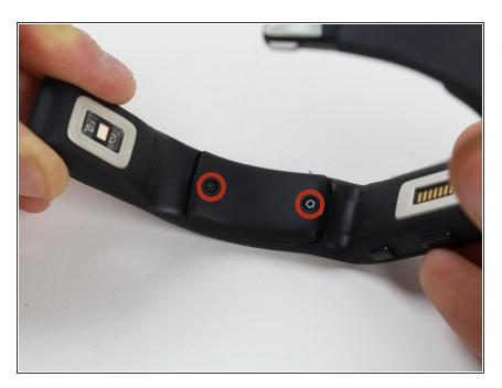
Unscrew both side panel 2mm screws using the T3 Torx screwdriver.
