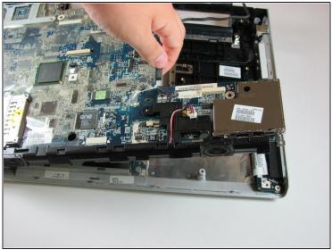
• Lift the system board off the computer frame.
