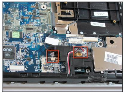
• Disconnect the USB audio cable and the modem cable.
