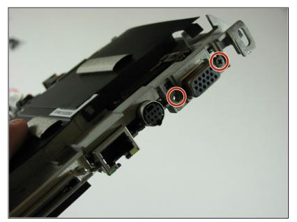
Remove the two 10.0 mm screws securing the fan on either side of the external monitor port.
