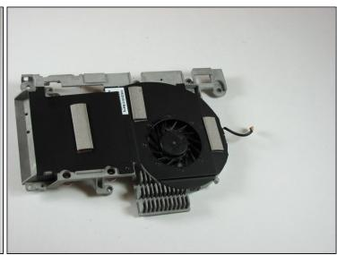
• Remove the fan from the computer frame.
