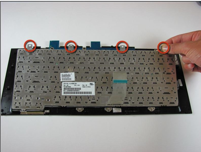
**i** This step is for replacing the keyboard only. If you are not replacing the keyboard, skip this step.
