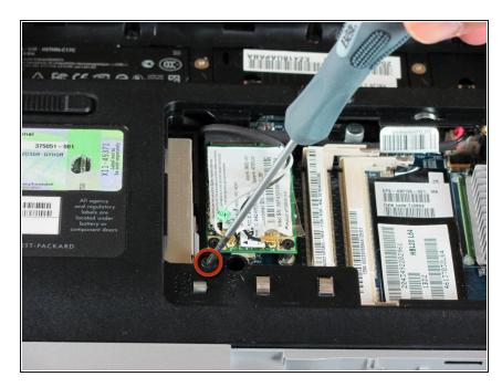
Remove the 11.0mm screw securing the optical drive to the computer.
