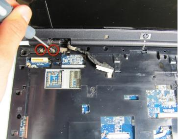
• Remove the four 7.0mm screws securing the screen to the computer.
