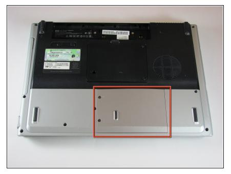
Locate the hard drive cover. Note that in this image, the RAM cover is still in place.
