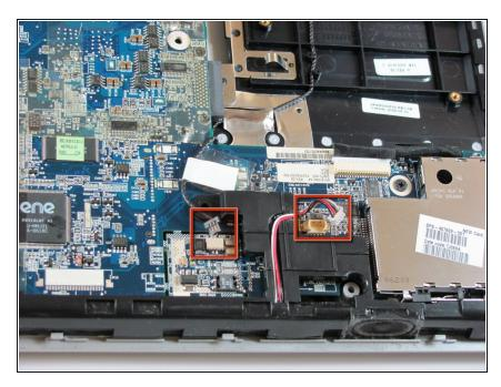
Disconnect the USB audio cable and the modem cable.
