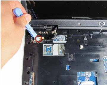
Use the plastic prying tool to disconnect the screen cable from the system board.
