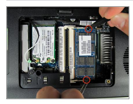
As in step 3, press the clips on both sides to release the second RAM clip.
