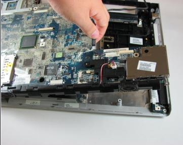
• Lift the system board off the computer frame.
