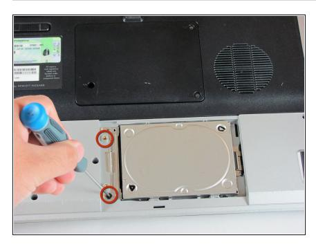
Remove the two 5.0mm screws securing the hard drive bracket.
