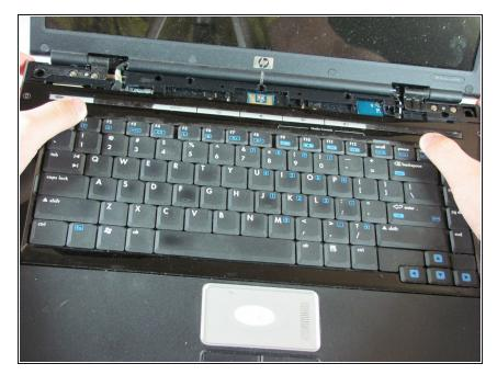
Next, remove the keyboard. Push on the keyboard frame above the function keys and slide the keyboard toward the screen.
