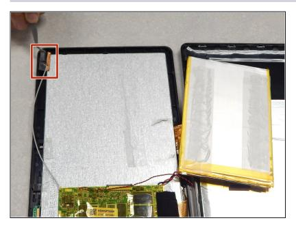
• Peel the WiFi antenna off of the monitor and move out of the way.
