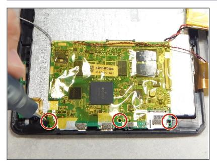
• Use a P00 Phillips screwdriver to remove the three screws securing the main-board to the back casing.
