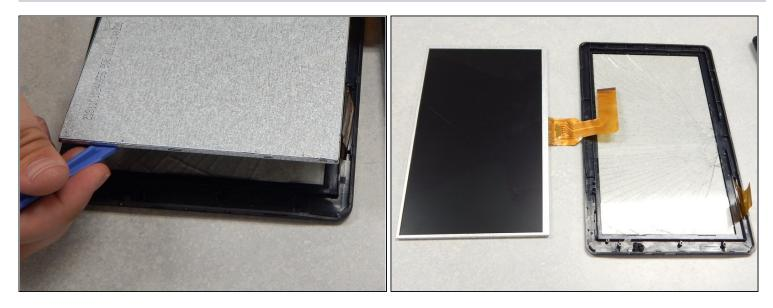
Use a separator tool to lift the screen from the port side of the casing and remove it.
