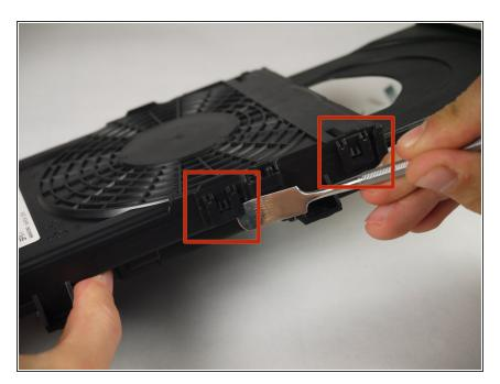
Insert the nylon or metal spudger under the clip and lift it up. There are 4 clips that need to be lifted, two on each side
