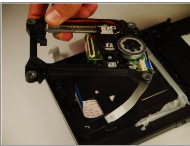
Carefully lift up the disc reader. It is still attached by a cable underneath!
