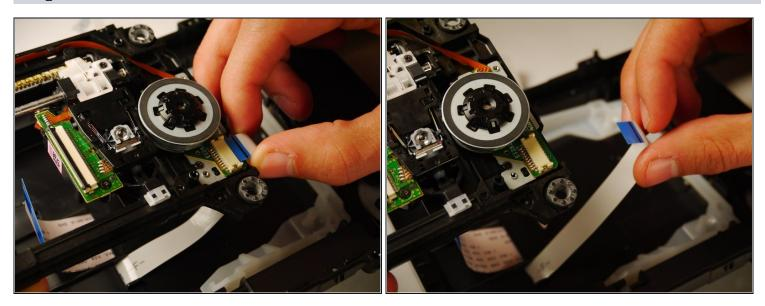
• Gently pull out the white 13 pin cable from the disc reader.
