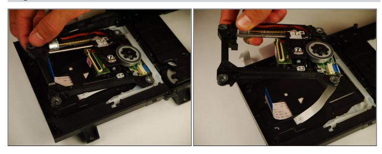
$\triangle$  Carefully lift up the disc reader. It is still attached by a cable underneath!
