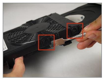
Insert the nylon or metal spudger under the clip and lift it up. There are 4 clips that need to be lifted, two on each side
