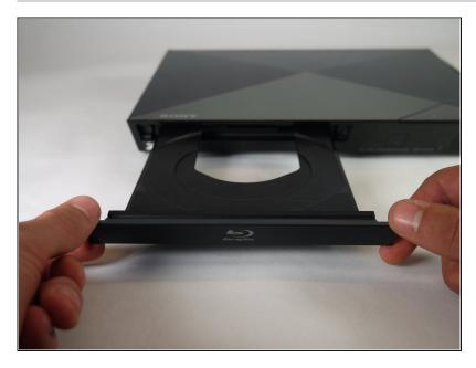
Grab the sides of the disc tray cover and carefully pull each side upwards, starting with the left side. This will unhook the cover from the tray.
