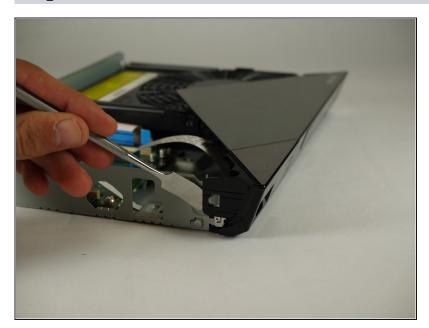
• Lift the clip on the opposite side of the device with the nylon or metal spudger.
