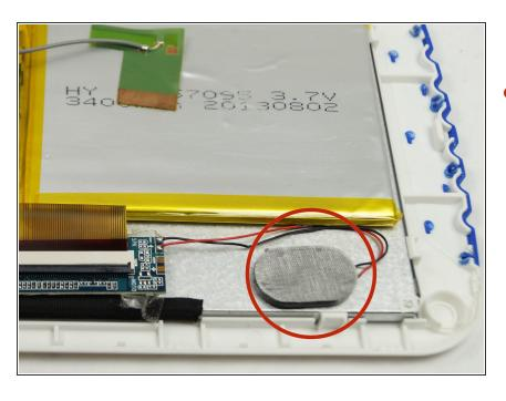
Locate the speaker on the back of the screen.
