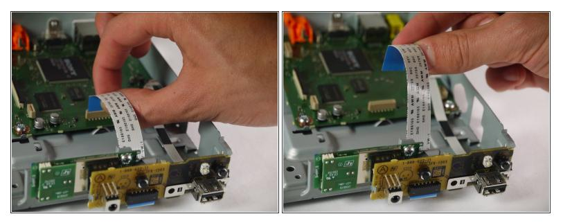
Mhen handling circuit boards like the motherboard and port board, make sure to only touch them on the sides.
