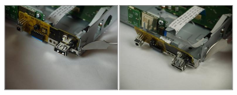
• Using the nylon or metal spudger, carefully unclip the port board from the side of the player.
