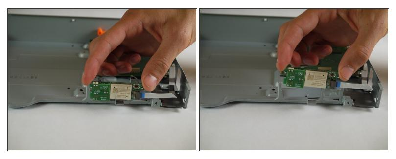
• Remove the Bluetooth module from the case.
