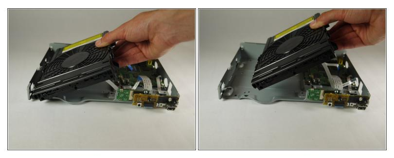
Slide the disk tray out from under the tabs on the case holding it down while lifting it out of the case.
