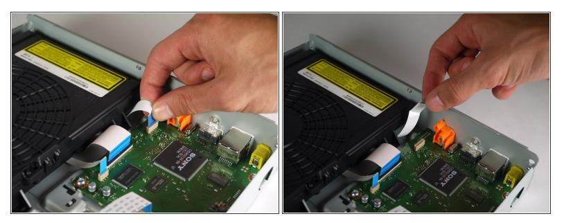
• Pull the medium-sized 9 pin ribbon cable out of its connector on the motherboard.
