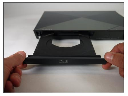
Grab the sides of the disc tray cover and carefully pull each side upwards, starting with the left side. This will unhook the cover from the tray.
