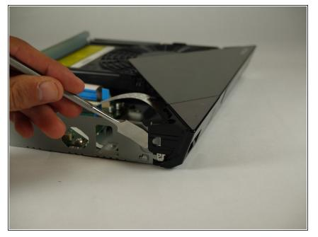
• Lift the clip on the opposite side of the device with the nylon or metal spudger.
