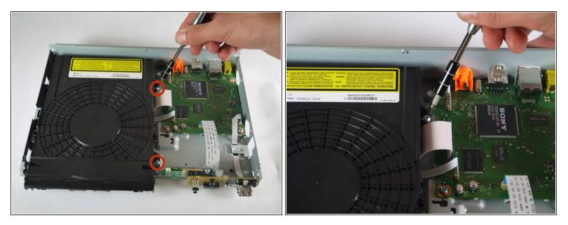
Using a Phillips #2 screwdriver, remove the two silver 8 mm screws on the right side of the disk tray.
