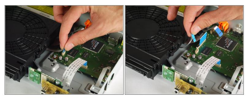
• Pull the small 5 pin ribbon cable out of its connector on the motherboard.
