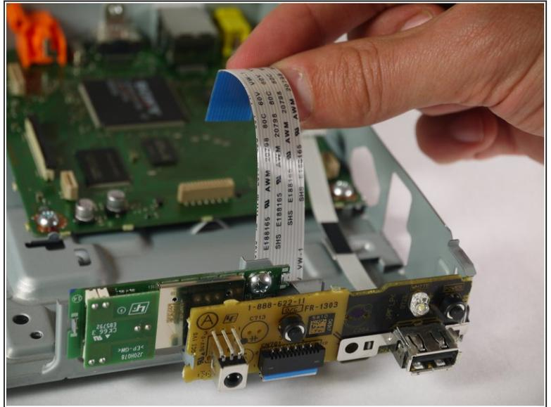
**!** When handling circuit boards like the motherboard and port board, make sure to only touch them on the sides.
