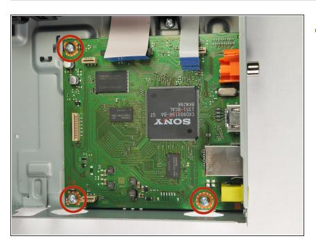
Remove the three screws holding the motherboard in the case.
