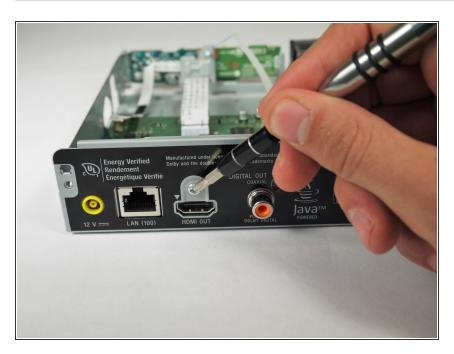
Remove the silver, 5 mm screw above the HDMI port with a PH2 screwdriver bit.
