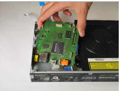
Mold the motherboard exclusively by its sides as to not short it out or damage it irreparably.
