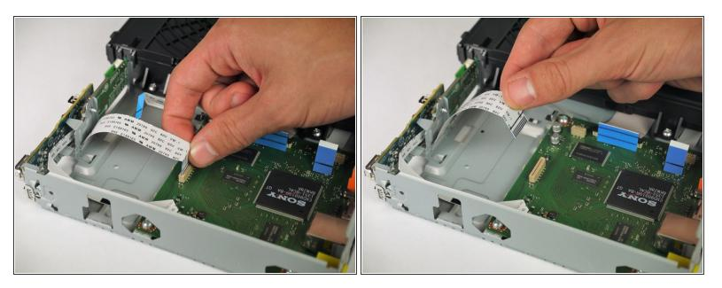
Remove the large, white ribbon cable connecting the motherboard to the port board (the larger of the two on the side nearest the front of the player) by lifting it out of its connector.
