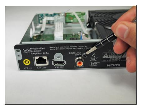
Remove the black, 1 cm screw to the upper right of the coaxial port using a PH2 screwdriver bit.
