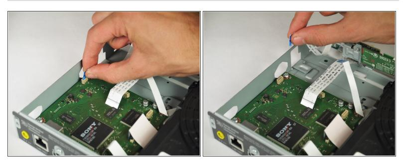
Lift up the white ribbon cable connecting the Bluetooth board to the motherboard (the smaller of the two on the front side of the motherboard) to remove it.
