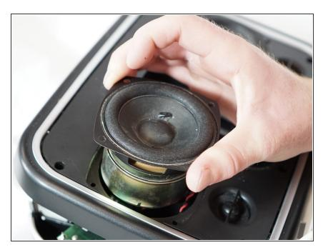
Take out the woofer from the front of the speaker with cable attached.
