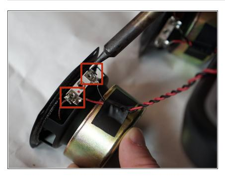
Desolder the cable from the woofer.
