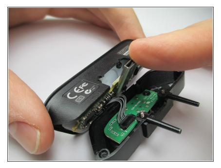
Pull back on the controller USB connector with your interview to separate the main adapter circuit board from the rubber mold in the button panel.
