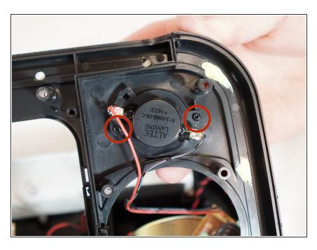
To fully remove the tweeter from the device, unscrew the two 7mm screws and the tweeter will be free.
