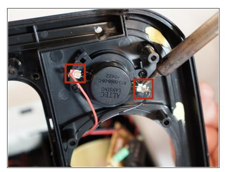
Remove the speaker cables by desoldering the two solder joints on opposite sides of the tweeter.
