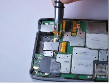
• Using a T5 Torx screwdriver, unscrew the two 4.0mm screws on the rear-facing camera cover.
