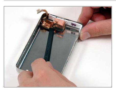
Slide a spudger beneath the orange headphone jack cable and use it to pry the cable up from the rear panel.
