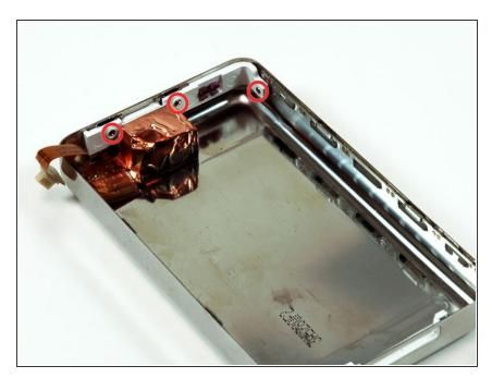
Remove the 3 silver Philips screws securing the headphone jack to the rear panel.
