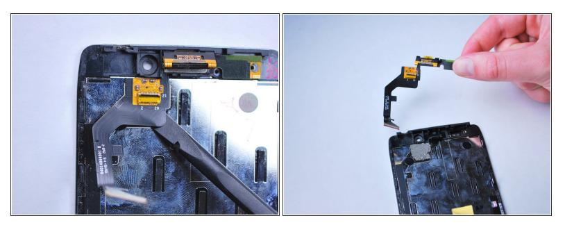
• Using a spudger, gently pry up on the lower right edge of the black earpiece speaker ribbon cable, attached to the screen, to release it from the LCD display.
