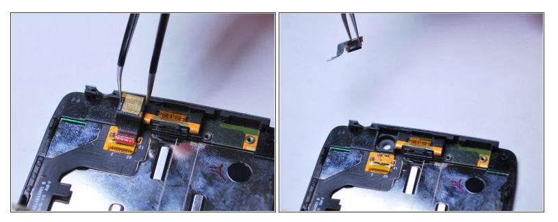
• Use tweezers to remove the front-facing camera by lifting it from the LCD display frame.
