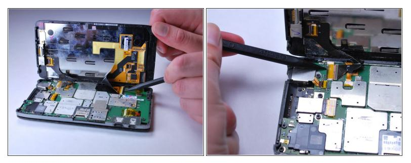
Release the two black ribbon flex cables by gently pulling up on the connection using the spudger.
