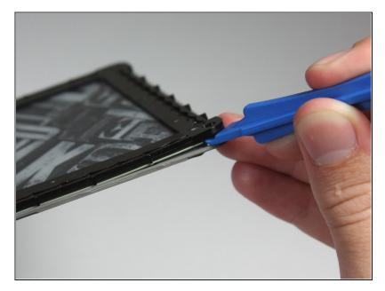
• Run the plastic opening tool around the edge to separate the bezel from the adhesive.
