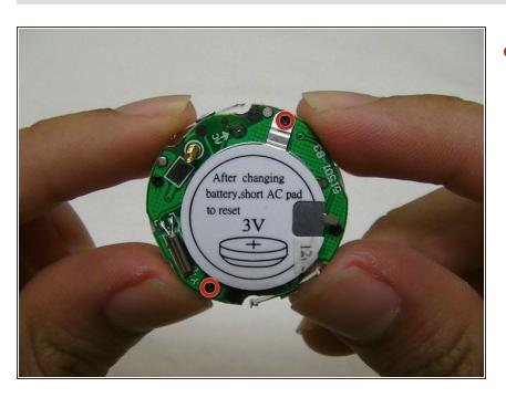
Remove two 1.5 mm Phillips Pan Head screws.
