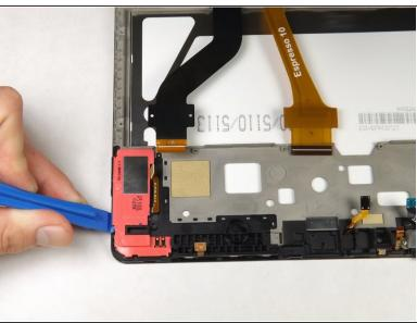
Using the plastic opening tool, gently pry the left speaker out of the slot and remove it
