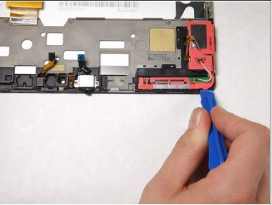
Using the plastic opening tool, gently pry the right speaker out of the slot and remove it
