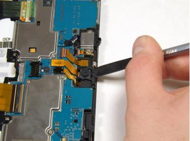
Gently lift the camera from its socket with the flat end of the heavy-duty spudger.
