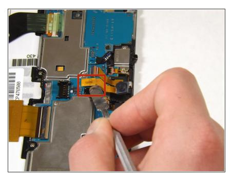
Gently lift the gold cable connector with the flat end of the heavy-duty spudger to disconnect it from the device.
