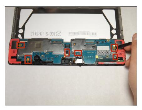
Use the flat end of the heavy-duty spudger to pop off and disconnect all the marked connectors attached to the motherboard.
