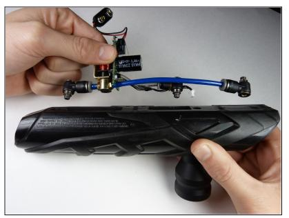
• Separate the solenoid from the gun's body by gently pulling it upwards.
