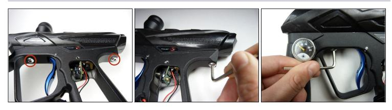
• Remove the front and rear 1" screws on the gun's grip frame using a 3/32" Allen Wrench.
