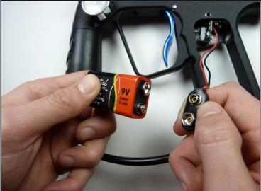
• Remove the 9V battery by unsnapping it.
