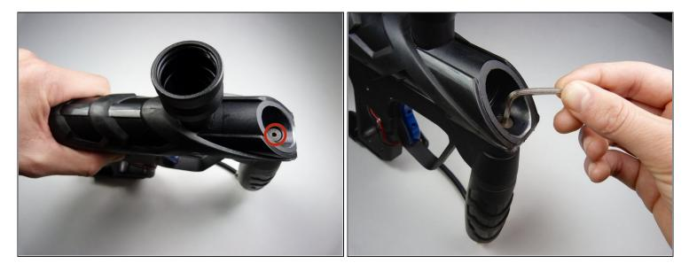
• Remove the 12 mm screw on the top of the grip frame using a 3/32" Allen wrench.
