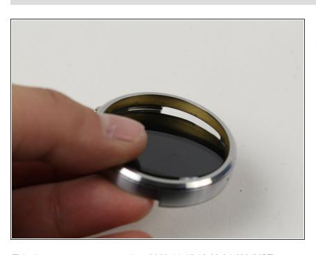
Slide the display out of the metal casing.
