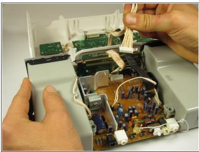
Unplug the narrow 9-pin connector from the motherboard.
