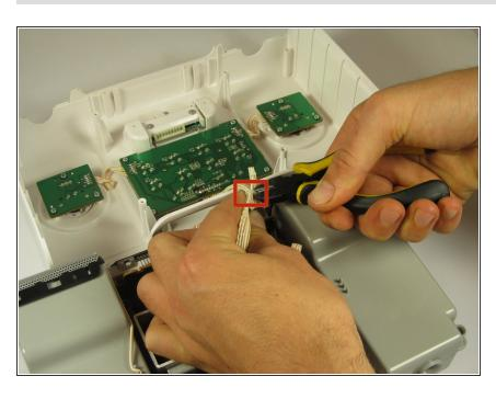
Cut the zip tie holding the wires together with a wire cutter. The two sides of the device housing are now fully separated.
