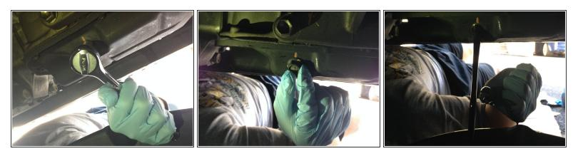
• Use the 14 mm socket wrench to loosen the oil drain plug. After a few turns, use your hands to loosen the plug until it is off.
