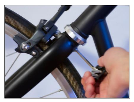
Using the 5mm allen wrench, check if the bolt on the backside of the caliper is snug.
