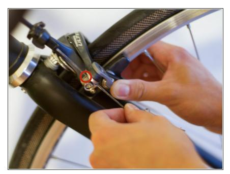
Check if your brake cable is inside the groove on the two plates (marked in the red cirlce) that hold the brake cable.
