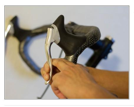
Check if the brakes are working properly by squeezing your brake levers.
