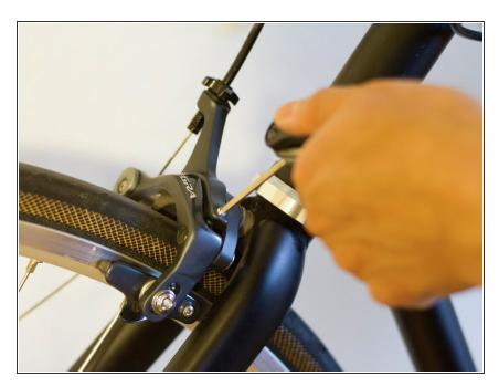
Make the brake pads equidistant from the rim by adjusting the tiny bolt on top of the caliper with a 3mm Allen wrench.
