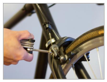
If your brake caliper is still tightened, loosen the cable bolt with a 5mm
