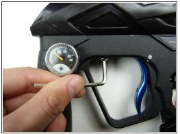
• Remove the front and rear 1" screws on the gun's grip frame using a 3/32" Allen Wrench.
