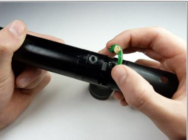
Remove the gun's green vision eye board by gently pulling it out using your index finger and thumb.
