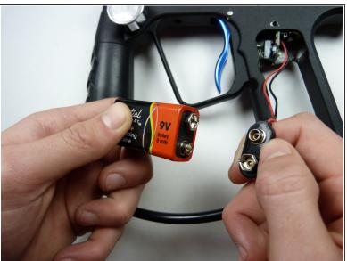
Remove the 9V battery by unsnapping it.
