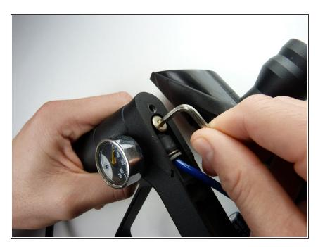
Remove the 1-1/4" screw that's attached to the blue tube above the front grip using a 3/32" Allen Wrench.
