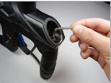
Remove the 12 mm screw on the top of the grip frame using a 3/32" Allen wrench.
