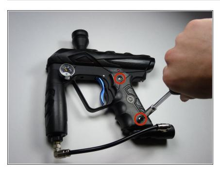
Remove the four 8mm screws on each side of the gun's grip using a Phillips #2 screwdriver.
