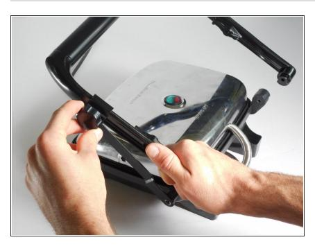
Unscrew the locking knob all the way to remove it.
