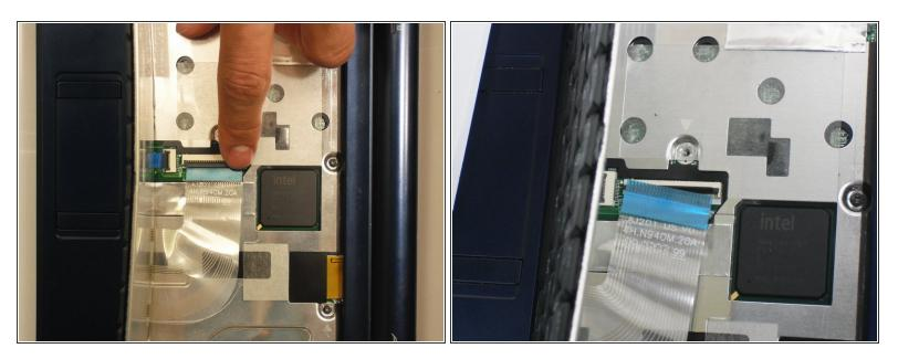
• Disconnect the ribbon by lifting the black plastic hinge and removing the clear blue cable.
