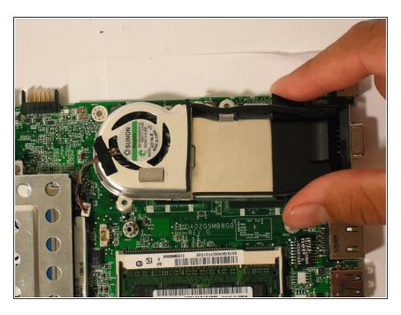
• Lift the fan housing from the motherboard.
