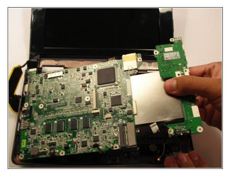
• Lift the entire motherboard assembly out the case.
