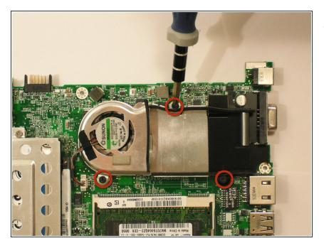
Remove the three 3.9mm screws using Phillips #1 screwdriver.
