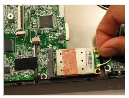
Disconnect the two antenna cables from the right side of the wireless card.
