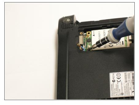
Remove the single 3.9 mm Phillips #1 screw from the bottom left of the wireless card.
