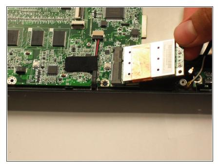
• Gently pull the wireless card to the right and slide it out of its socket.
