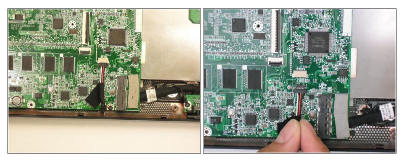
• Disconnect the speaker cable from its socket on the motherboard.
