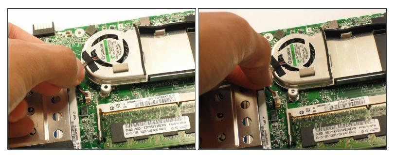
• Disconnect the fan cable from the motherboard.
