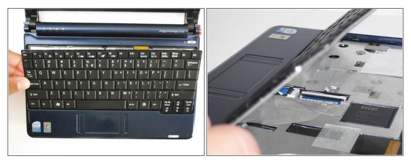
• Lift top of keyboard up. If it doesn't lift easily, there may be tabs on the sides - use the tool to ease them aside and/or shift the keyboard from side to side.
