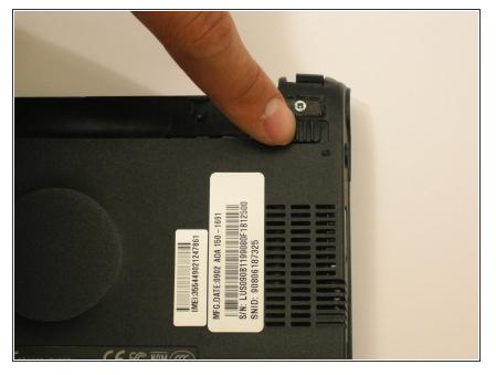
Slide the latch located on the opposite hinge from the lock while pushing the battery up.
