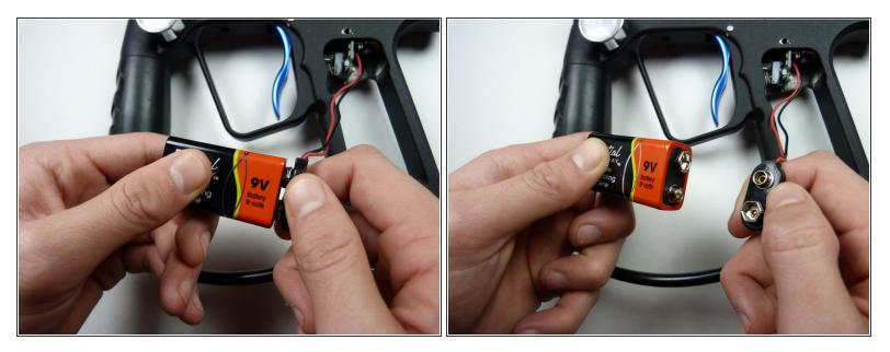
• Remove the 9V battery by unsnapping it.
