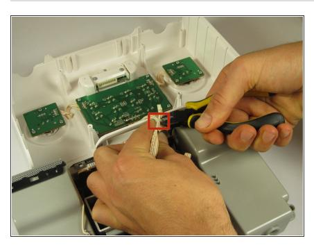
Cut the zip tie holding the wires together with a wire cutter. The two sides of the device housing are now fully separated.
